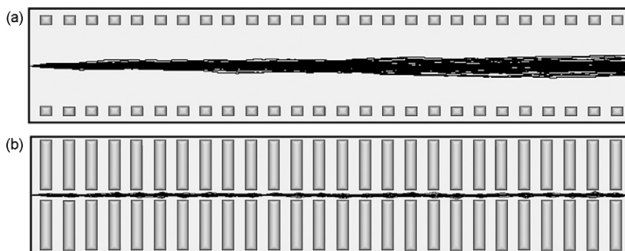
Fig. 1. Longitudinal cross-sections of uniform field (a) and periodic-focusing field (b) IMS drift tubes showing ion trajectories in black. Ion transmission is increased in the PDC IG via the periodic-focusing mechanism which confines ions near the central drift axis and maximizes ion transport through the exit of the drift tube.
